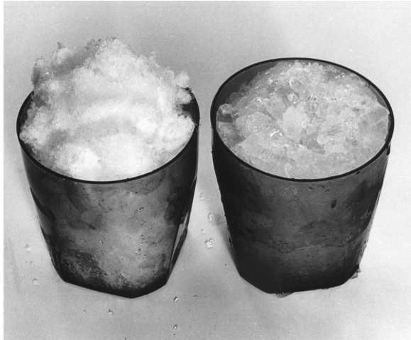
Figure 2. Shaved ice, with frosty ice on the left and ice after slushing on the right.
