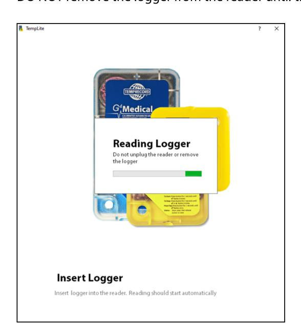
When the logger has been read, EXCEL and PDF documents will be generated. (At this stage, it is safe to remove the logger.)
